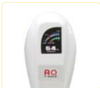
LED Display: shows speed and battery status
